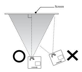
If this unit is not placed parallel to the screen, the projected image is distorted in the shape of a keystone.
