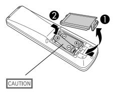
Check the positions of the (+) and (-) marks inside the battery holder to ensure the batteries are inserted the correct way.
